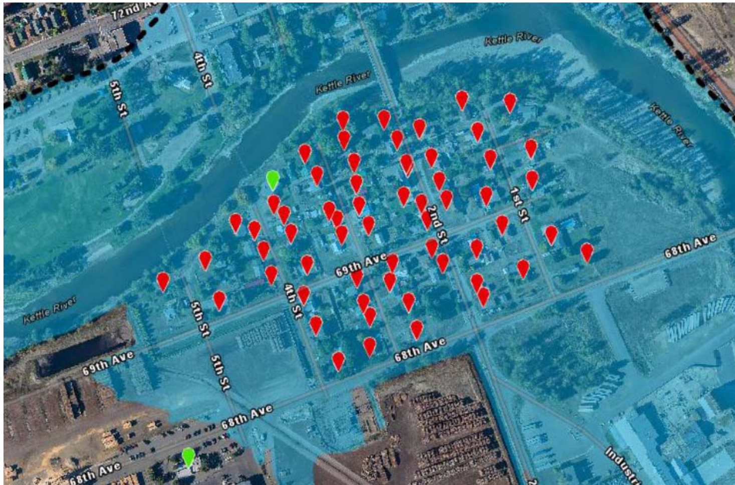
Figure 10 – City of Grand Forks North Ruckle Neighbourhood [Green=not damaged; Yellow=limited damage; Red=moderate-severe damage]
